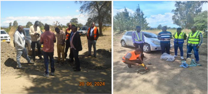
Plates 1: Site inspection and field density test at Mbalizi Road section
